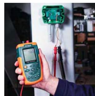
SOURCE DE PRÉCISION POUR L'ÉTALONNAGE DES APPAREILS DE PROCESSUS.
