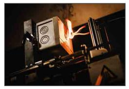
**Glow wire resistance, climatic chamber** And many more tests.
