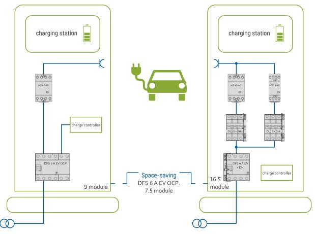
power supply with short-circuit back-up fuse
