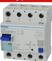
AC/DC sensitive type B, for installations with frequency inverters, UPS devices etc, increased surge-current resistant, short-time delayed, lightning resistant, fire prevention up to 150 kHz, for special voltages 500 V
