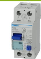
AC/DC sensitive, for heat pumps, increased surge-current resistant, short-time delayed, fire protection according to VDE 0100-420
