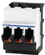
*empty housing with 40-mm adapter for track mounting with fitted cartridge up to 63 A, without fuse plug and fuse*
