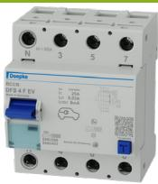
sensitive to residual currents Type F, short-time delayed, lightning resistant, with DC tripping threshold 6 mA, for electromobility
