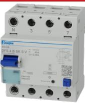
AC/DC sensitive type B, for installations with frequency inverters, UPS devices etc, increased surge-current resistant, lightning resistant, selective, for special voltages 500 V
