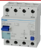
AC/DC sensitive type B, for installations with frequency inverters, UPS devices etc, increased surge-current resistant, short-time delayed, lightning resistant
