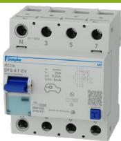
sensitive to residual currents Type F, short-time delayed, lightning resistant, with DC tripping threshold 6 mA, for electromobility, for harsh environments
