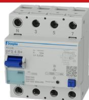
AC/DC sensitive type B+, for installations with frequency inverters, UPS devices etc, increased surge-current resistant, short-time delayed, lightning resistant, fire prevention up to 20 kHz
