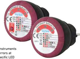
The Testavit Schuki 1 A and 3 A socket outlet testers are essential test instruments for all professional tradesmen. They indicate all hazardous connection errors at sockets, cable drums and connection cables in 230 V installations via specific LED combinations. This enables the quick and safe checking of installations. The Testavit Schuki 1A is also fitted with an FI/RCD test circuit.
