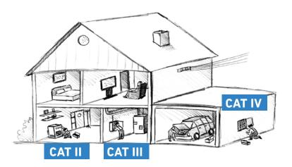
Measuring instruments are classed in accordance with 3 different categories that indicate the ranges for which they are approved:
