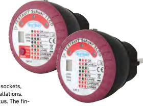
The Testavit Schuki 1 LCD and 3 LCD enable everyone to check easily if sockets, cable drums or connecting cables are correctly connected in 230 V installations. Three LEDs permit quick and clear determination of the connection status. The finger contact enables testing for the presence of impermissibly high contact voltage at the protective earth connection. The Testavit Schuki 1 LCD can also be used to trigger a 30 mA FI circuit breaker (RCD).
