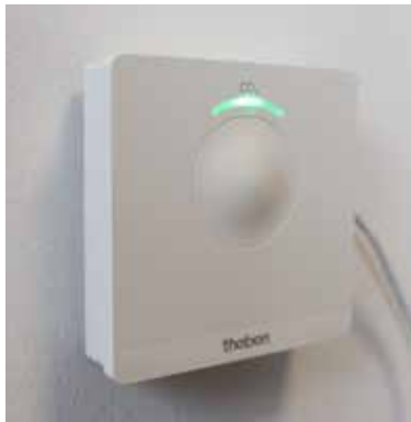
LED light system on the AMUN 716 CO 2 Monitor
