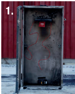
1. A lithium battery was placed at the bottom of the cabinet and the MAUS unit/units were placed at the top.
