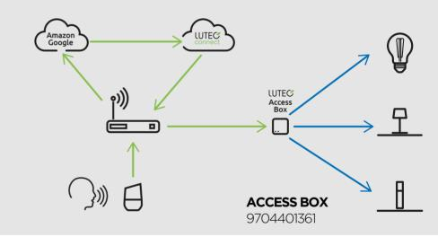
Via Cloud access you can control all the devices in your LUTEC Connect lighting network from anywhere out of home.
