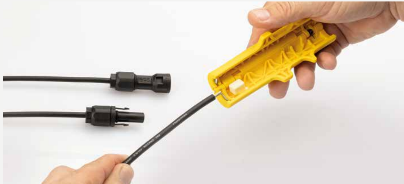
Length stop 8.5 and 15 mm, for connecting common PV plugs
