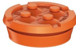
Double membrane seals made of elastic plastic with two sealing membranes, max. four cable entries for control cables, f. wall thicknesses 1.5 - 4.5 mm, thermoplastic elastomer, orange
