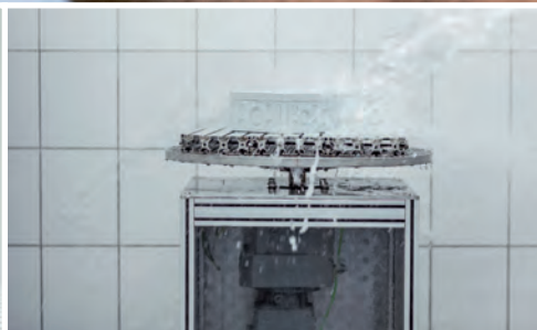
Water protection testing
