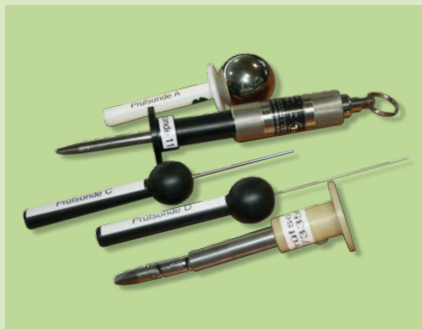
Test probe according to DIN 60529
