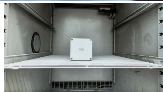
Air conditioning cabinets tested to -30 degrees
