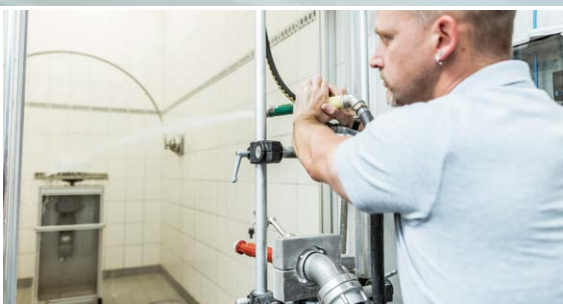
Water protection testing
