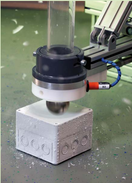
The splinters are ice residue from the cooling process at -35^{\circ}\text{C} .
