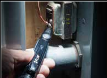
High sensitivity mode is useful for working on low-voltage systems
