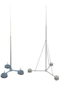
Self-supported aluminum termination rods with hinged tripod made in galvanized steel and adjustability up to 10° inclination. Dimensioned to withstand winds up to 145km/h. Includes concrete weights, roof protection plates and clamp for connection with round conductor Ø 6/10 mm.
