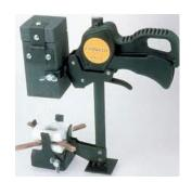
Cadweld Multi combining a versatile mould with a set of ceramic tissue gaskets that allow different types of welds among round conductors up to  $\emptyset$  10 mm, with flat conductors up to 30 x 3.5 mm and with grounding electrodes up to  $\emptyset$  17.2 mm without changing the mold in each connection type.
