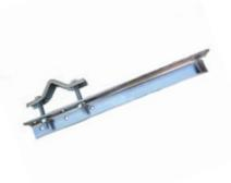
Light anchorage to be embedded into the wall. Manufactured in "L" shaped profile of  $30 \times 30 \times 3$  mm.
