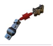
Spark gap for equipotential bonding to connect aerial mast with the protection system. With plastic coating and protection degree IP 65. Includes stainless steel connectors for connecting with masts  $\emptyset$  30 to  $\emptyset$  50mm and round conductors  $\emptyset$  8 to  $\emptyset$  10 mm and flat up 30 mm.
