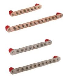
Equipotentiality bonding bars to attach to the wall using thermoset insulators, self-extinguishing, halogen-free and resistant to ultraviolet rays. With screw connection system stainless steel M-10, which allows the union of conductors of different types and sections through appropriate terminals.
