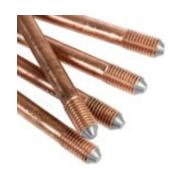
Threaded grounding extensible electrodes. With 254 $\mu$  copperbond steel for conducting grounding. With electrolytic copper coating of 254 $\mu$ , 99.9% purity and extremely high quality, which provides a high degree of corrosion resistance. Possibility to get greater lengths by using the accessories required for its extension and sunk.
