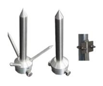
With adapting piece made of brass/aluminum and stainless steel flange for outside connection with masts until Ø 55mm with round conductor up Ø15mm and flat conductor up to 50 x 5mm.
