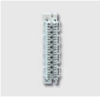
AsLe A 10 LSA-Plus* 260 006 ● Terminal strip with LSA-Plusterminals; 10 pairs; 96 mm fixing gap; light grey (similar RAL 7035); 26 x 105 x 22 mm; 97 g
