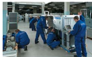
AirVents air handling unit workshop
