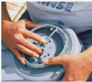
Clip the front ring onto the housing.
