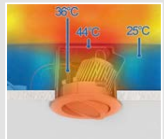
Temperature profile pivoting 5W built-in spotlight
