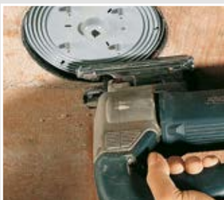
Open front part using a fretsaw.
