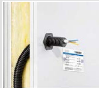
Wall entry with M16-M25 combination entry, in plaster-board fire-protection wall with M25 conduit.
