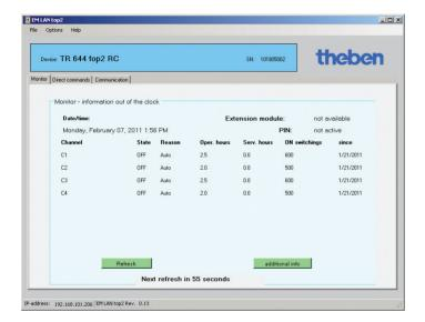
The status information from the connected time switches appears in the **Monitor** register; e.g. Date/time, upgrade module, channel, PIN, On switching times etc. (see fig.).
