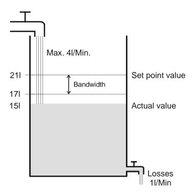
A filling volume of 15l gives rise to a control deviation of 211 - 151 = 61Because our actual value lies outside the bandwidth, the control will control the flow at 100% i.e. at 41 / minute
